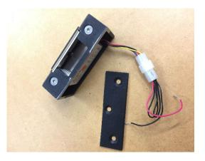
Install the 3mm stainless steel TSMB onto the door frame. Then install the electric strike plate with the 2 x 5mm stainless steel screws provided. There are 2 x cable exit slots to suit different application.
